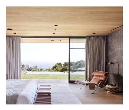
MADERA Pine core Panels are intended for application on walls + ceilings and can be specified in fixed lengths up to twenty feet. They're made with 2mm thick natural oak sawn lamellas in various grades up to fifteen inches wide on a Pine core. Wall + ceiling panels feature a custom tongue and groove profile for easy installation, and are available in all Madera finishes, various dimensions, and multiple grades.
