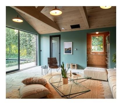
MADERA MDF core Panels are intended for application on walls and ceilings and can be specified in fixed lengths up to fourteen feet. Made with natural oak veneers in various grades up to twelve inches wide on a MDF core. Wall and ceiling panels feature a custom tongue and groove profiled for easy installation, and are available in all MADERA finishes, various dimensions and multiple grades.
